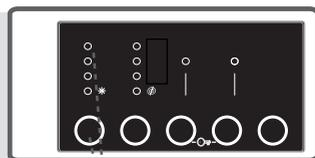
When you select a new programme, there won't be any display on the temperature adjustment leds on the display panel. When you press the temperature adjustment button, the max. temperature value of the programme you have selected shall appear on the led display panel.
