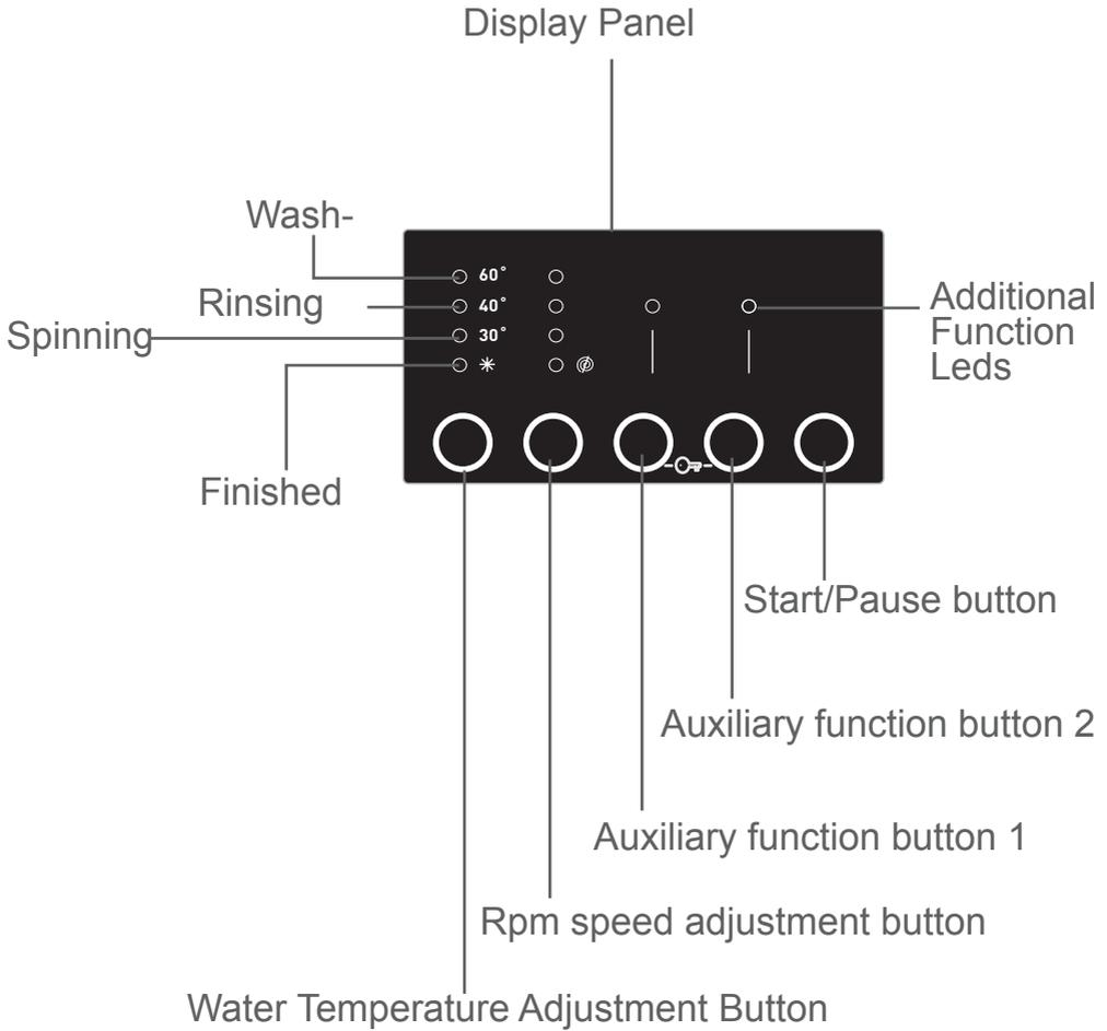
On the display panel, you can see the washing water temperature of your machine, speed setting of your machine, the auxiliary functions you have selected and the stage of the programme you are running on your machine (⏸ pre wash/wash state, 🧼 rinsing stage, 🌀 spinning stage).
