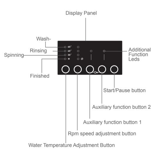
On the display panel, you can see the washing water temperature of your machine, speed setting of your machine, the auxiliary functions you have selected and the stage of the programme you are running on your machine (山 pre wash/wash state, 螢 rinsing stage, ③ spinning stage).
