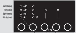
You may make the programme active by pressing the cold washing button on the display panel when the led light of the \* symbol turns on.
