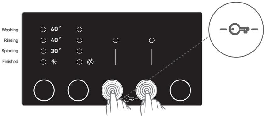
If pressed any button while child lock is active, the Additional Function Leds will blink on the display.
